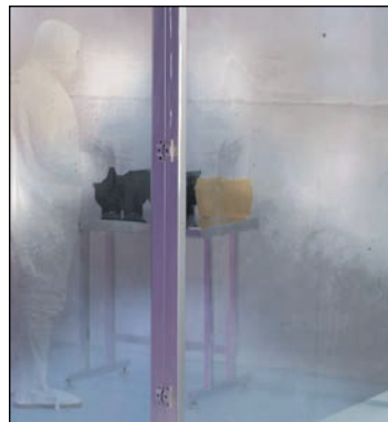
The surface of anti-static PVC can bloom over time and develop a viscous coating, requiring periodic cleaning.
